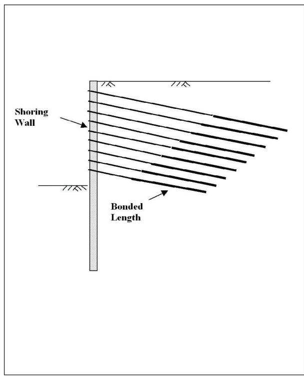
Figure 6-10: Basic Components of a Tieback Anchor
