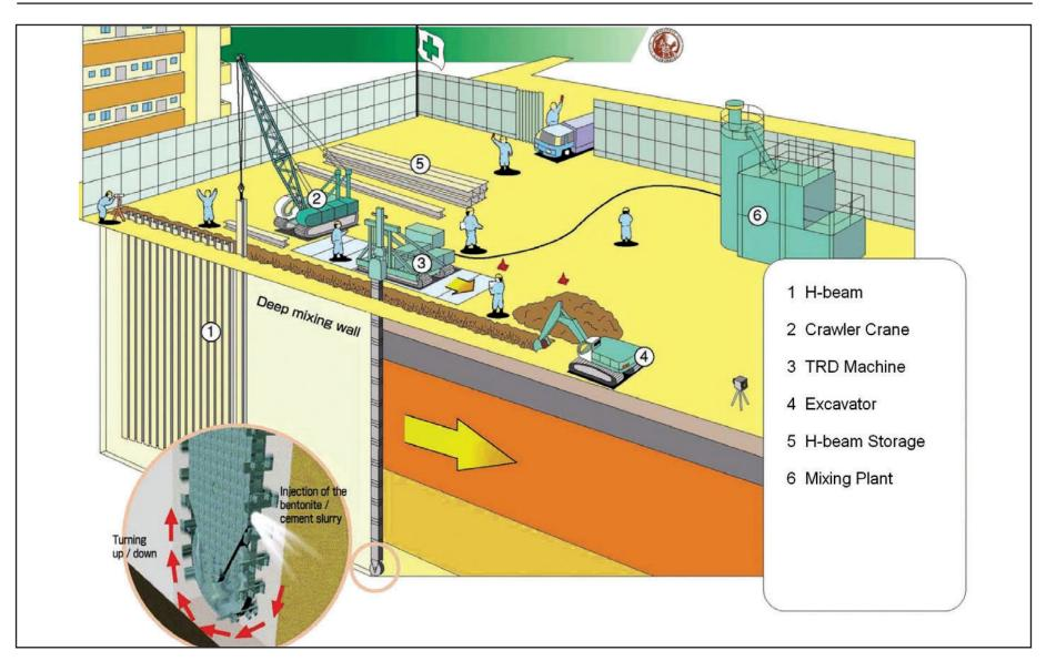
Figure 6-18: Trench Remixing and Deep-Wall Method (TRD)
