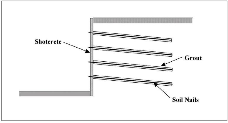
Figure 6-12: Soil Nail Wall
