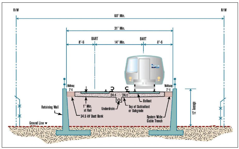
Figure 6-4: Retained Fill Guideway
