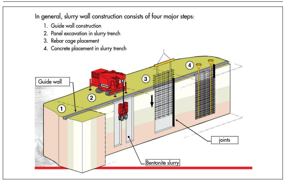
Figure 6-19: Construction of a Diaphragm Slurry Wall
