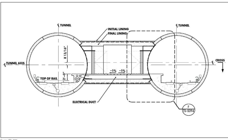
Figure 6-27: Cross-Passage Connecting the Tunnel Bores
