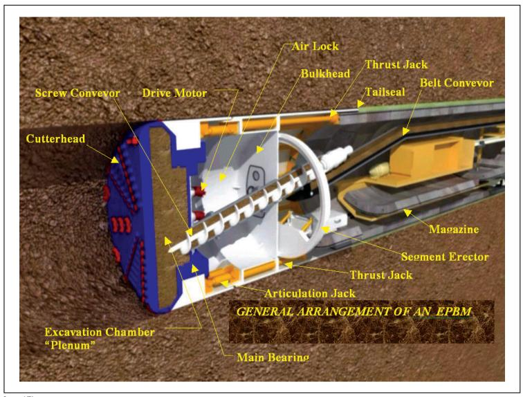
Figure 6-23: General Arrangement of an Earth Pressure Balanced Tunnel Boring Machine
