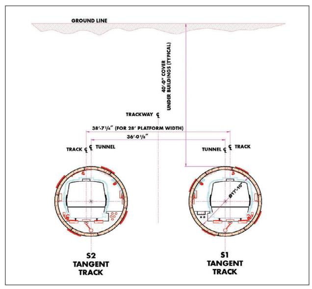
Figure 6-20: Diameter and Spacing of Tunnel Bores (TRD)
