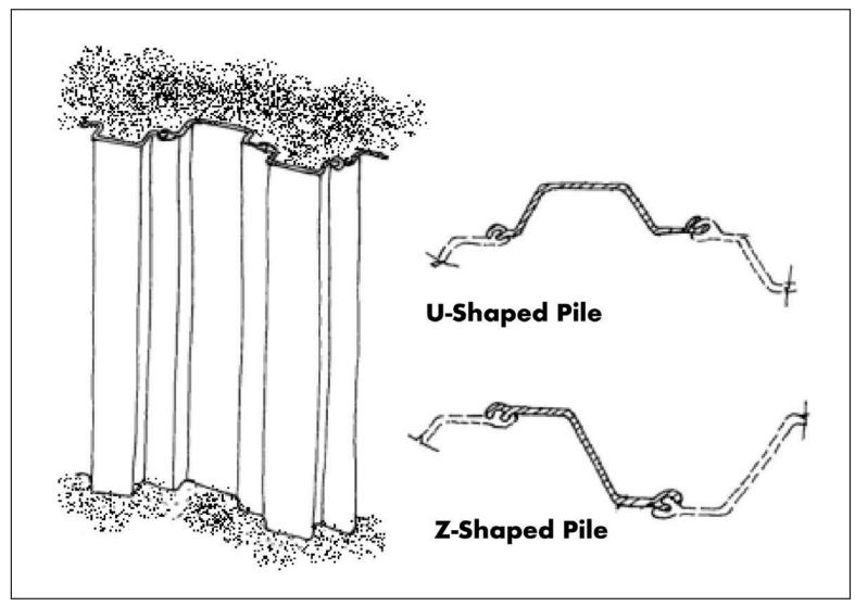
Figure 6-8: Steel Sheet Pipes
