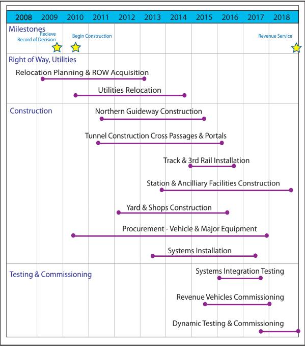
Figure 6-2: SVRTP Alternative Proposed Construction Schedule
