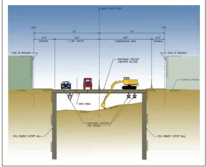
Figure 6-14: Ongoing Excavation After Temporary Deck Installation
