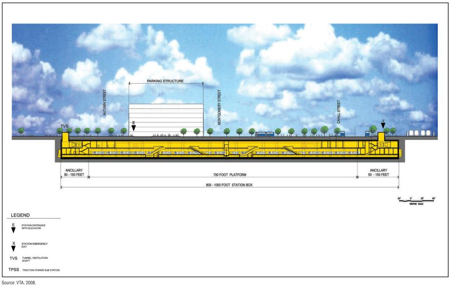
Figure D-17: Diridon/Arena Station Conceptual Longitudinal Section A-A Looking South **SVRTP Alternative Only**
