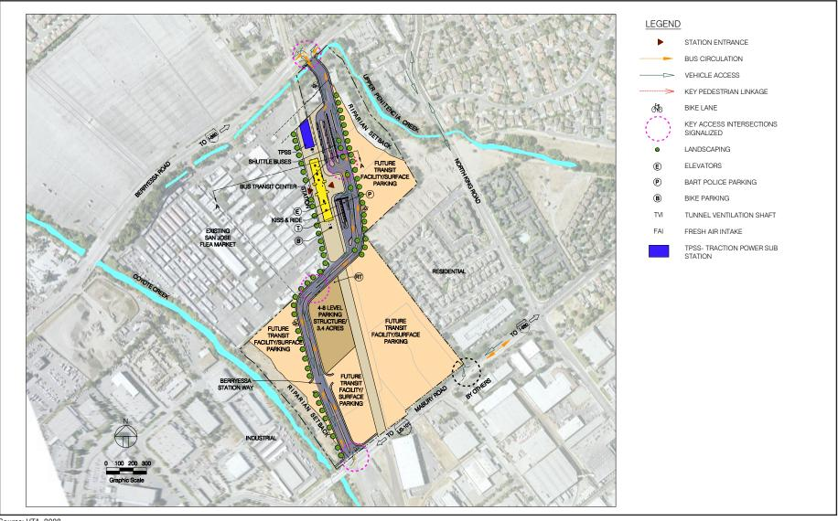
Figure D-7: Berryessa Station Conceptual Site Plan **BEP and SVRTP Alternatives**
