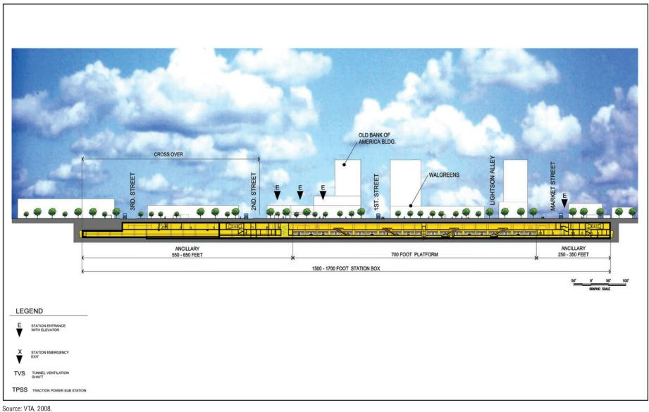
Figure D-14: Downtown San Jose Station Conceptual Longitudinal Section A-A Looking South **SVRTP Alternative Only**
