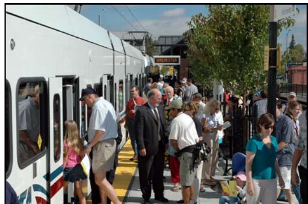
Low Floor Vehicles Provide Level Passenger Boarding
