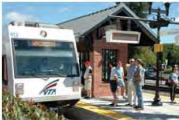
Low-floor light rail vehicles and retrofitted platforms provide fast, level boarding for all riders
