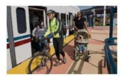
Low-floor light rail vehicles and retrofitted platforms provide quick, level boarding for all riders.
