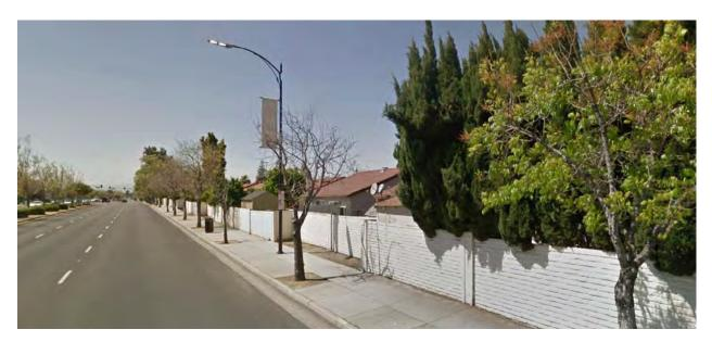
Figure 24: Placement of roadway light fixtures along the back of sidewalk requires wheel chair users to meander around light fixtures and tree locations
