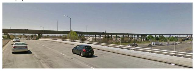
Figure 19: Roadway light fixtures spaced far apart likely provide insufficient light for pedestrians to feel safe
