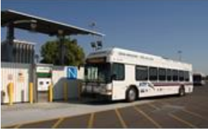
Zero-Emission Bus (ZEB) at hydrogen fueling station
