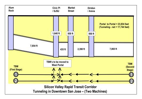
Figure 4.19-16: Tunneling Two Directions (Two TBMs)
