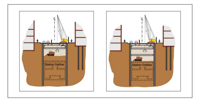
Figure 4.19-13: Station Construction Below Deck
