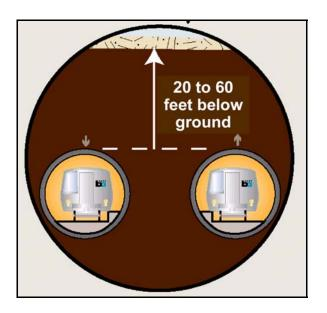
Figure 4.19-7: Conceptual Cross Section for BART Alternative Tunnel
