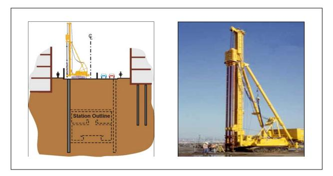
Figure 4.19-11: Construction of Outside Protective Walls
