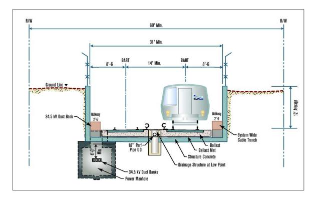
Figure 4.19-4: Conceptual Retained Cut Cross Section for BART Alternative
