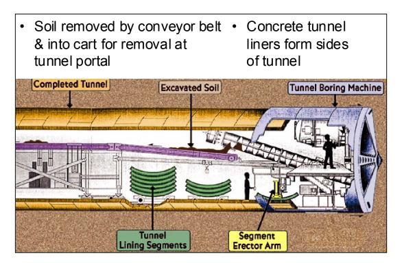
Figure 4.19-8: Earth Pressure Balance Tunnel-Boring Machine
