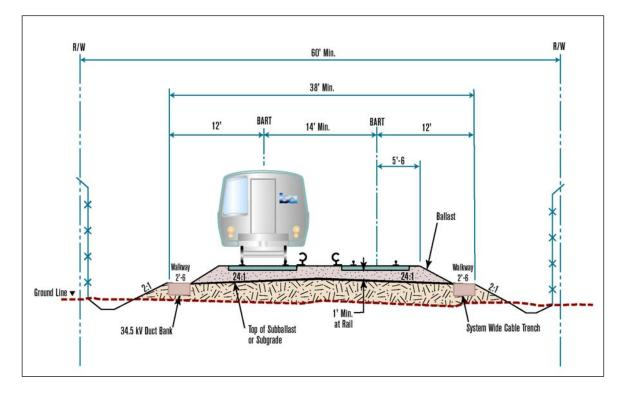
Figure 4.19-1: Conceptual At-Grade Cross Section for BART Alternative
