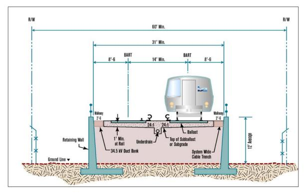
Figure 4.19-2: Conceptual Retained Fill Cross Section for BART Alternative
