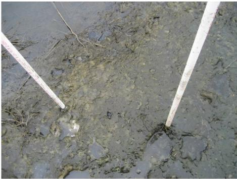
**Photo B-5.** Feldspar sedimentation plot; white feldspar is buried beneath a layer of new sediment.
