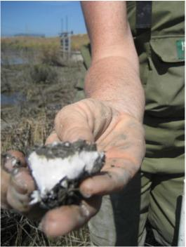
**Photo B-6**. Feldspar sample cut from sedimentation plot showing a layer of sediment above the white feldspar marker horizon.
