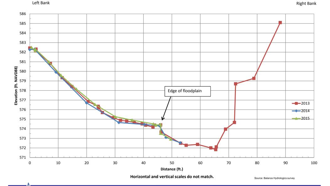
Figure 31 . Cross section 101, Alum Rock WY2015 monitoring, Santa Clara County, California.
