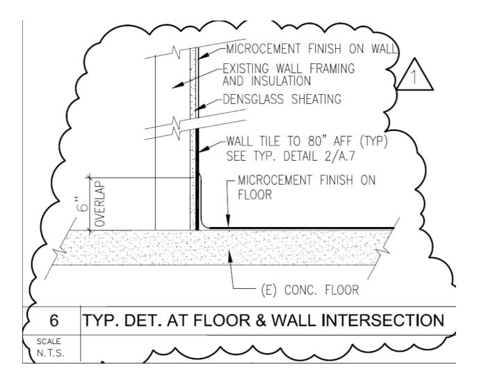
A36. Restrooms - All walls (except Storage Room) – floor to 80" AFF to be finished in tile. Remaining wall above the tiles to be finished in Microcement. Ceiling to be painted.
