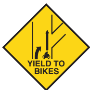
ADVANCE OF ON-RAMP VTA SW-2
